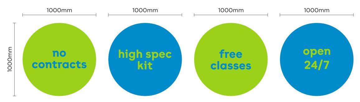
4-OFF illuminated suspended roundels. Fabricated from aluminium signcase, 100mm deep with removable frames, painted blue/green. Fitted with vinyl decorated acrylic face panels. Illuminated via white LEDs.
