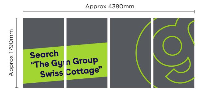
Grey background vinyl with suma cut green vinyl 'Super g' applied to the window areas. Sizes taken from elevation drawing, survey required for accurate sizes.
