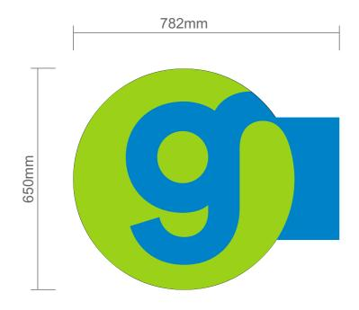
3-OFF aluminium projecting sign painted PMS 279C, fitted with fully illuminated acrylic face panels c/w translucent green vinyl. Internally illuminated via LEDs.
