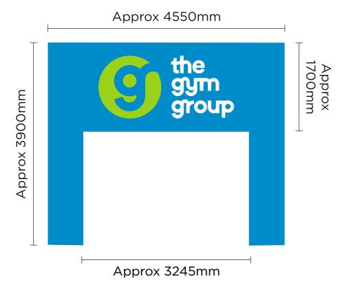
Folded aluminium panel finished Blue PMS Process Blue, stencil cut to accept logo and text backed with opal acrylic. Green translucent vinyl externally applied to the 'g' logo. Internally illuminated via white LEDs.
