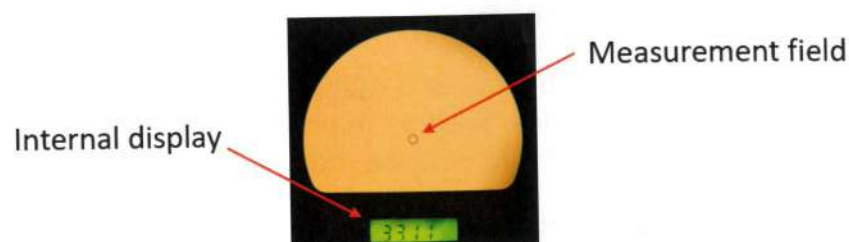
Figure 12.1: View through a luminance meter showing the measurement field
