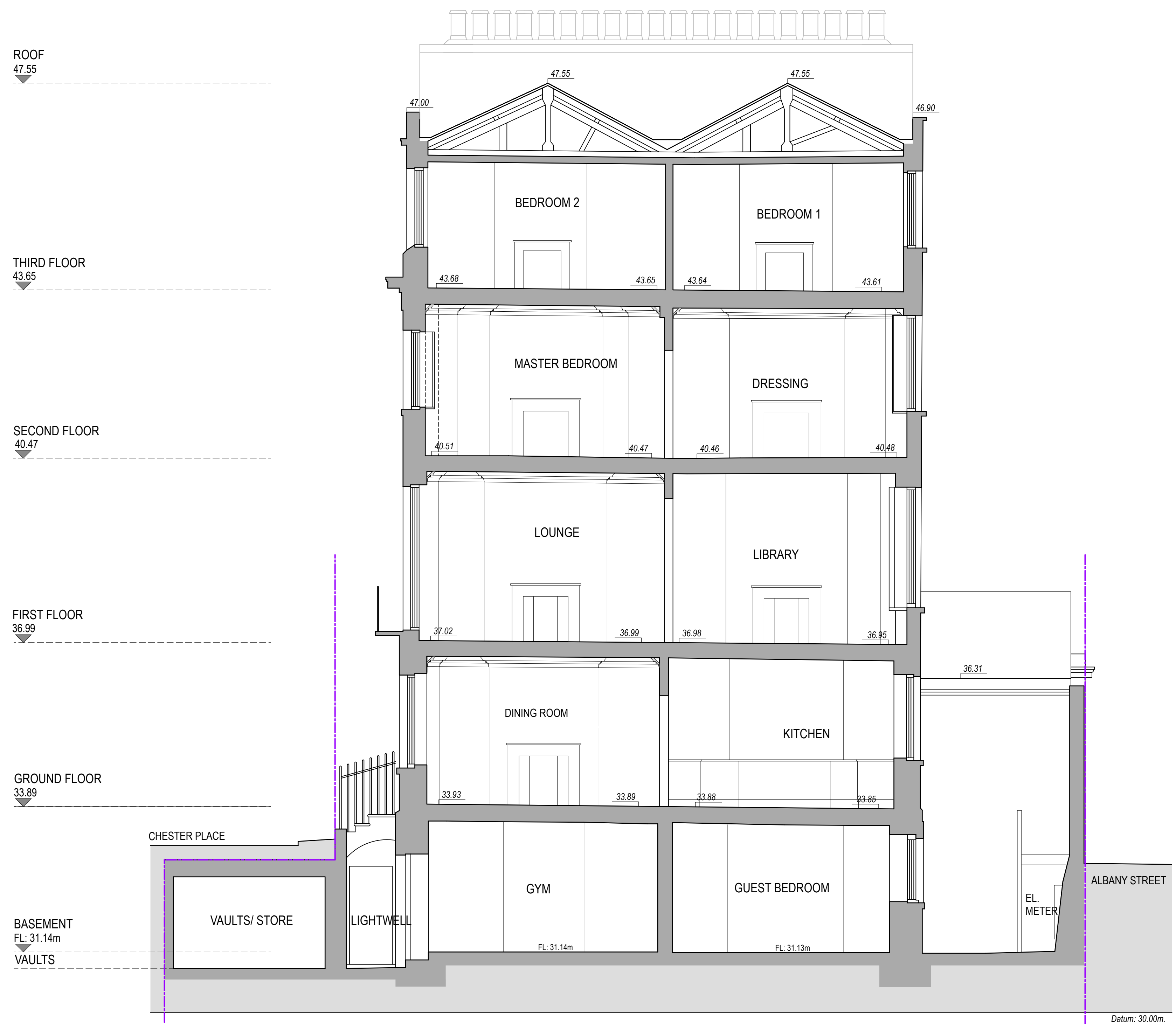
SECTION A-A ON SECTION OVERVIEW
