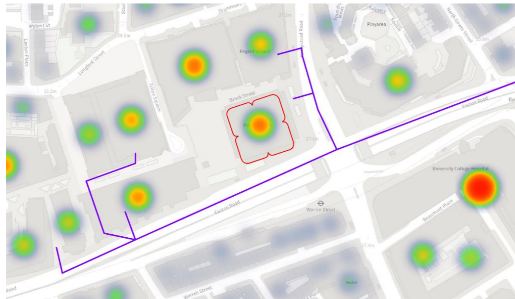
Figure 10: Image from the London Heat Map showing the proposed Euston Road heat network
