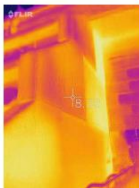
Figure 4.2 - Rear of block A showing the heated party wall from the coils and the unheated wall
