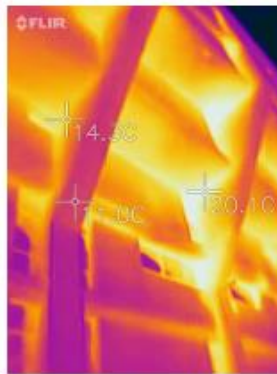
Figure 4.2 - Rear of block A showing the heated party wall from the coils and the unheated wall
