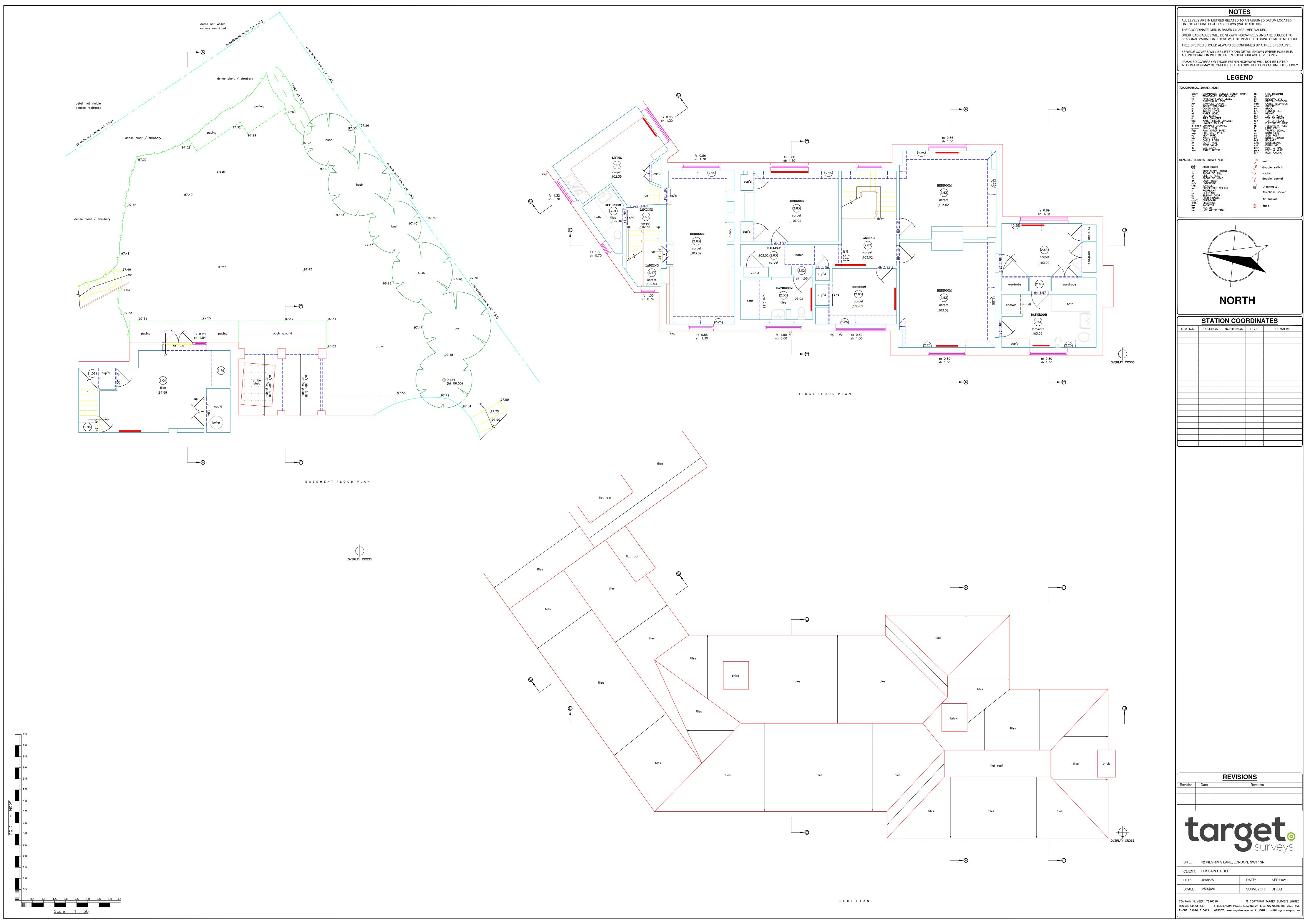
ALL LEVELS ARE IN METRES RELATED TO AN ASSUMED DATUM LOCATED ON THE GROUND FLOOR AS SHOWN (VALUE 100.00m). THE COORDINATE GRID IS BASED ON ASSUMED VALUES. OVERHEAD CABLES WILL BE SHOWN INDICATIVELY AND ARE SUBJECT TO SEASONAL VARIATION. THESE WILL BE MEASURED USING REMOTE METHODS.
