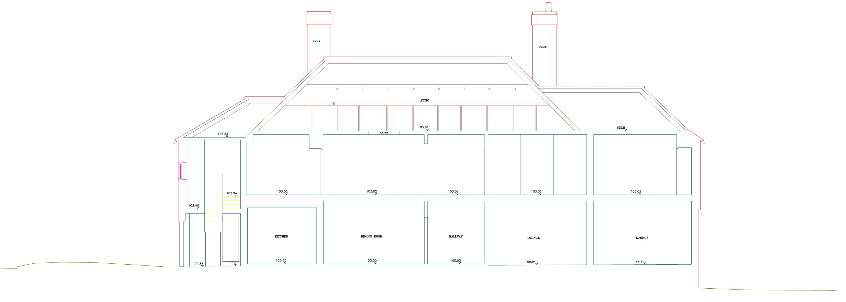
Datum 96.00m SECTION B-B ALL LEVELS ARE IN METRES RELATED TO AN ASSUMED DATUM LOCATED ON THE GROUND FLOOR AS SHOWN (VALUE 100.00m).
