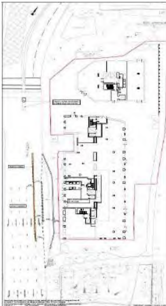
Fig. 7 – Construction Phase - Bus stop D replaced by "Pit Lane" - Bus Stop B enhanced - Jersey barrier and traffic cones installed - A41 part lane closure to allow safe entry / exit to site
