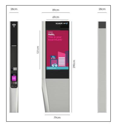
The Dimensions of the proposed replacement BT Street Hub 3 are also shown below: 2986mm (h) x 1236mm (w) x 350mm (d)
