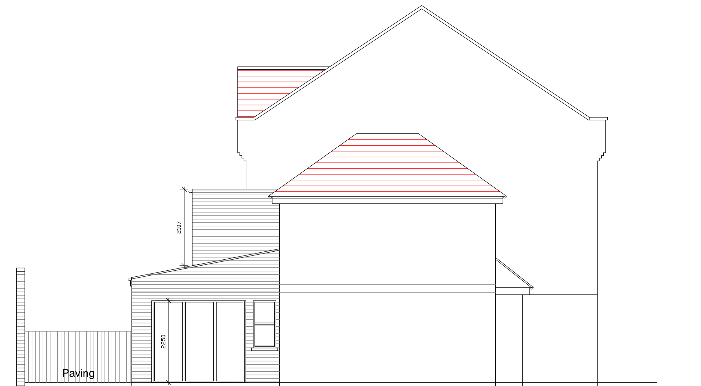
EXISTING SIDE ELEVATION
