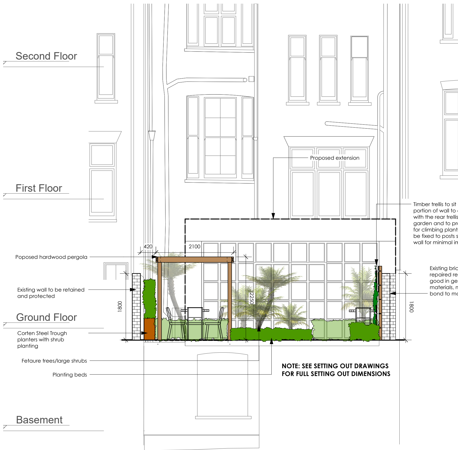
1 ELEVATION A-A - VIEW LOOKING BACK TO BUILDING/PROPOSED EXTENSION 1:50@A3
