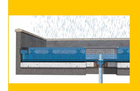
I lue roof attenuation technology is proposed to store rainfall under permeable paving on the roof to allow a controlled means of discharge.
