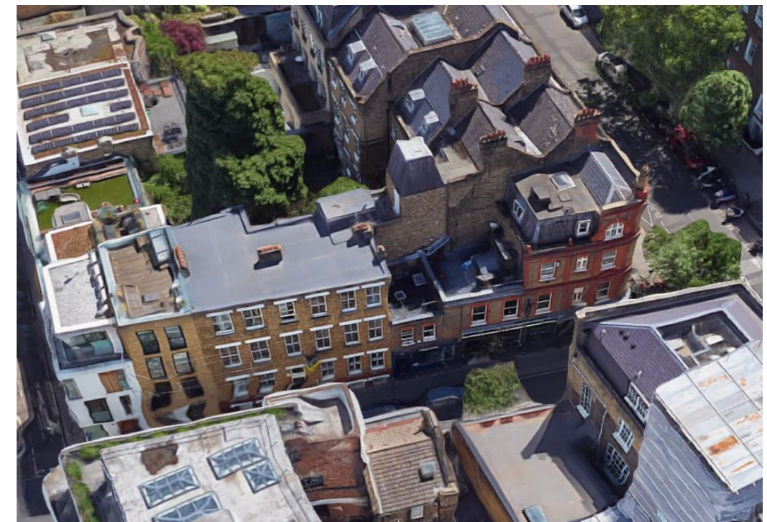
Figure 18: An aerial view of the site looking south showing the link block rising above the original darkened yellow stock brick of the northern flank of the site.
