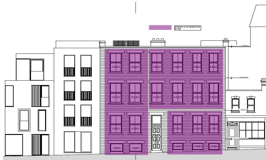
Figure 5 Front Elevation showing windows to be replaced.
