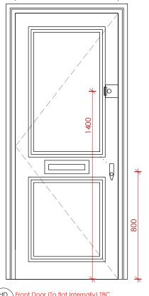
HD Front Door (To flat Internally) TBC V01.1 Ahmarra Blenheim 2A 2 Panels or similar to be approved by KLD, painted in Farrow and Ball Wevet No. 273, Estate Eggshell Flat (FP) Panel styles, APM 1 Moulding profile 30min Fire rated
