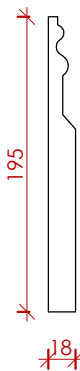
701 Skirting board 2nd Floor Master Bed, Bed 2 Bathroom, WC All 3rd Floor Painted in Farrow and Ball Wevet No. 273, Estate Eggshell 1 : 5
