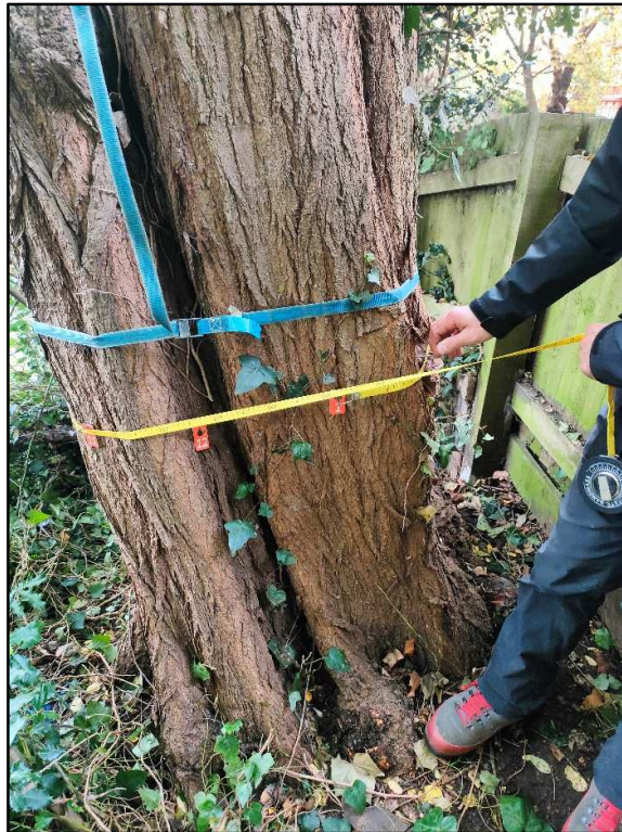
Figure 5: Image of PiCUS Test Plane conducted on Robinia
