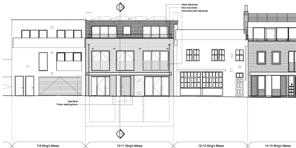
Figure 1 – The proposed front elevations for 10-11 King's Mews (ref: 2017/4543/P) demonstrating the mansards characteristic of King's Mews.
