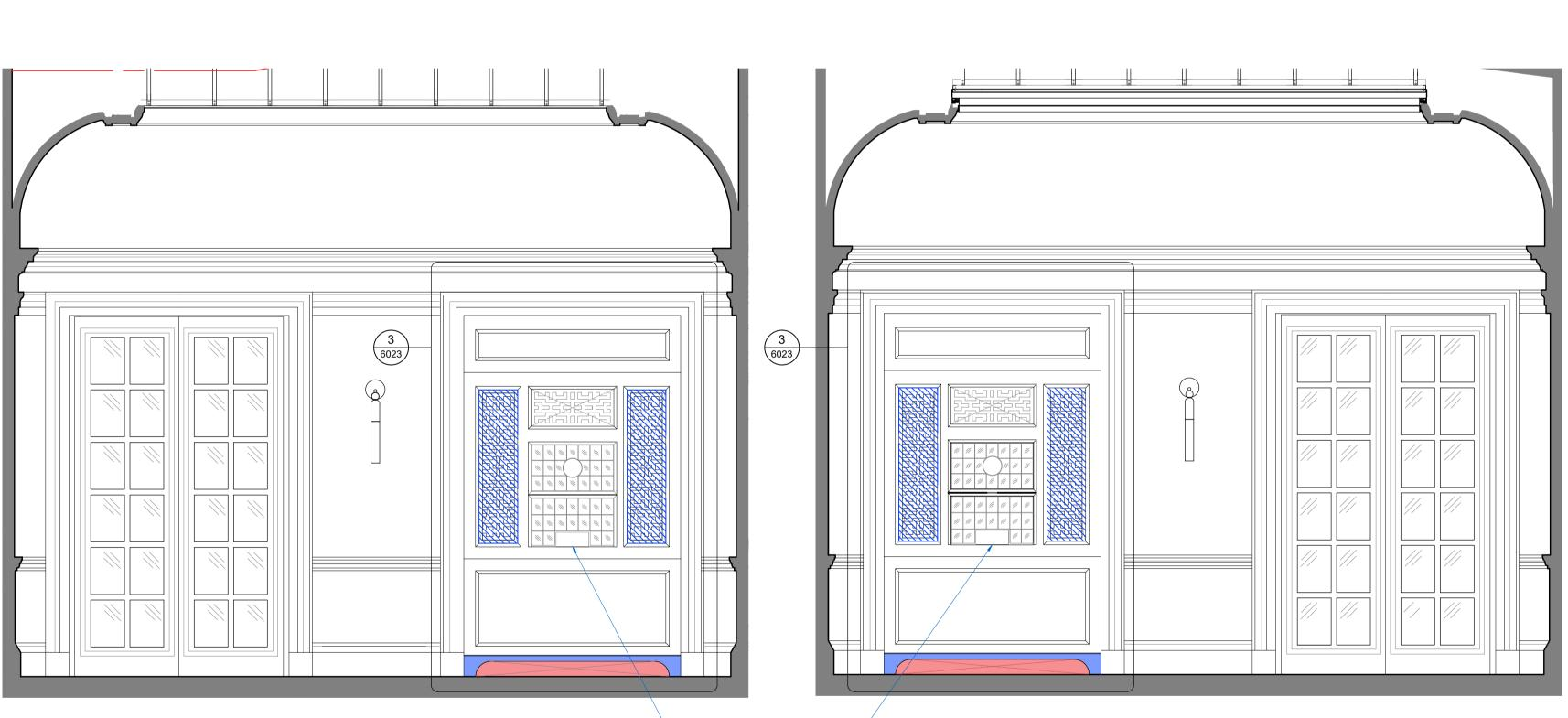
New services riser to be installed within previous West ticket office, and new ventilation duct to be installed within previous East ticket office. Original features within G.45 to be retained. Careful repairs to existing ticket booths, timber and glazing panels.
