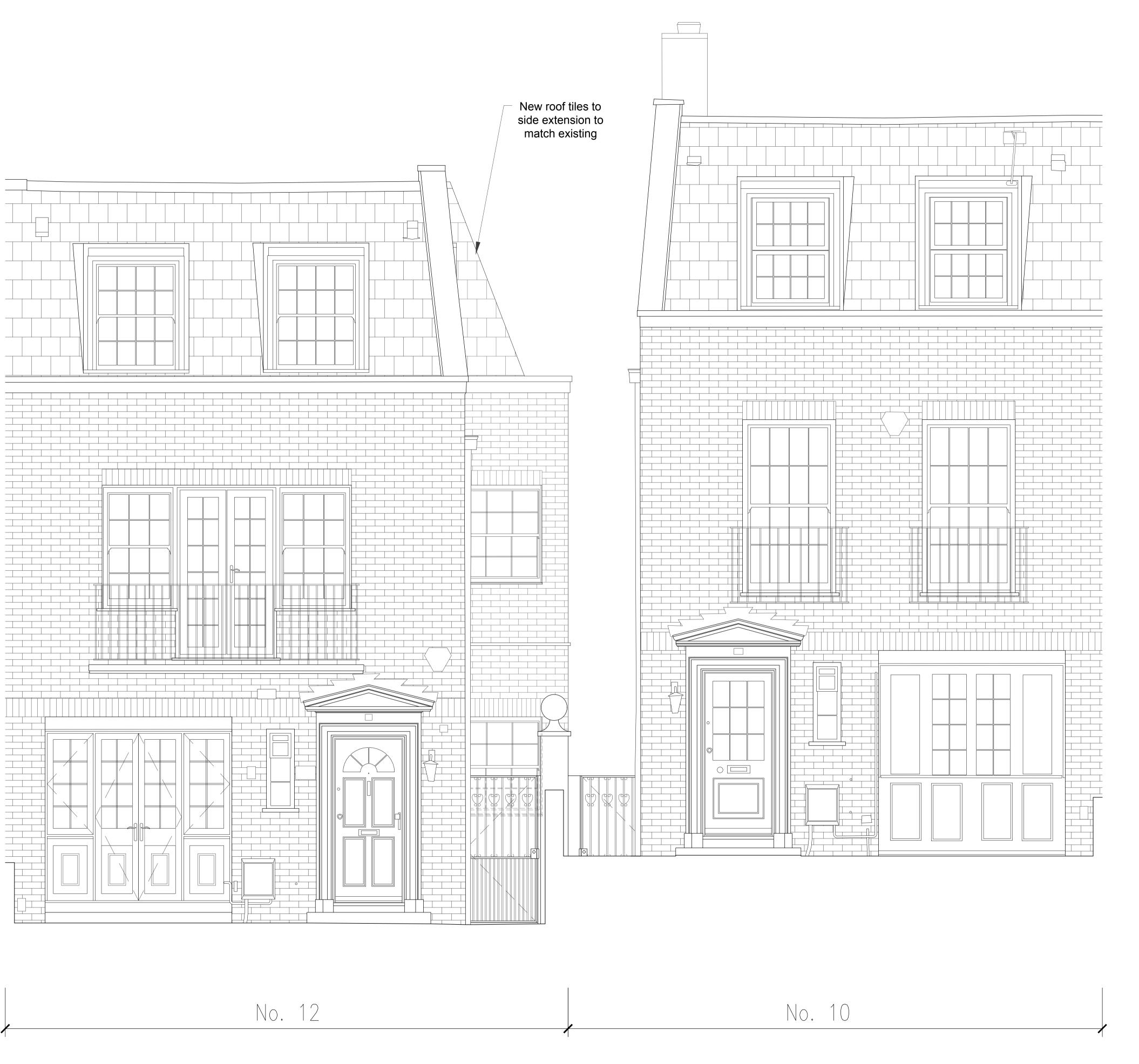
Proposed Front | South Elevation Scale 1:100 @ A3 | 1:50 @ A1
