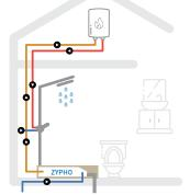
**3.** The preheated water is transferred to the boiler only.
