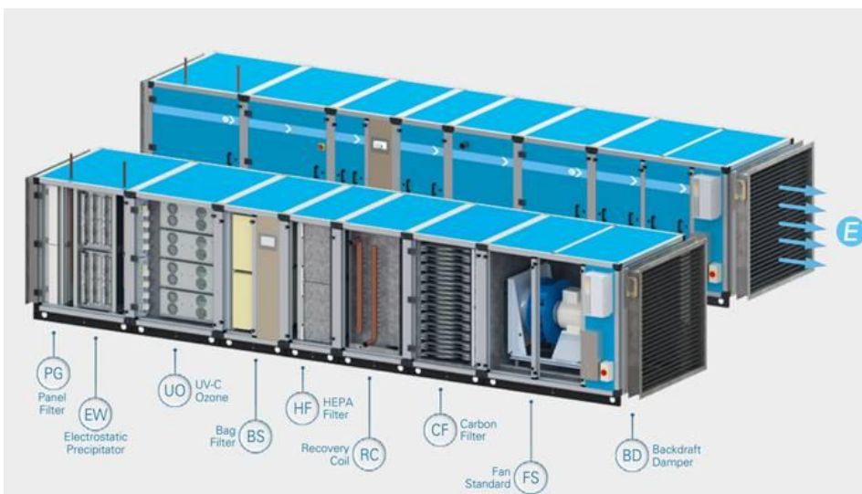
Figure 3: Typical kitchen extract air handling unit configuration
