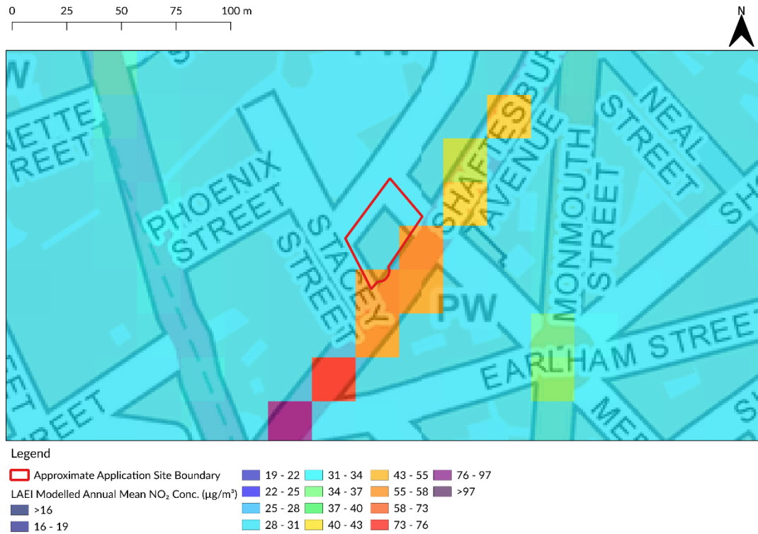
Figure 5: Modelled 2025 annual mean concentrations of NO 2 (GLA, 2023). Contains OS Data © Crown Copyright and Database rights 2024.
