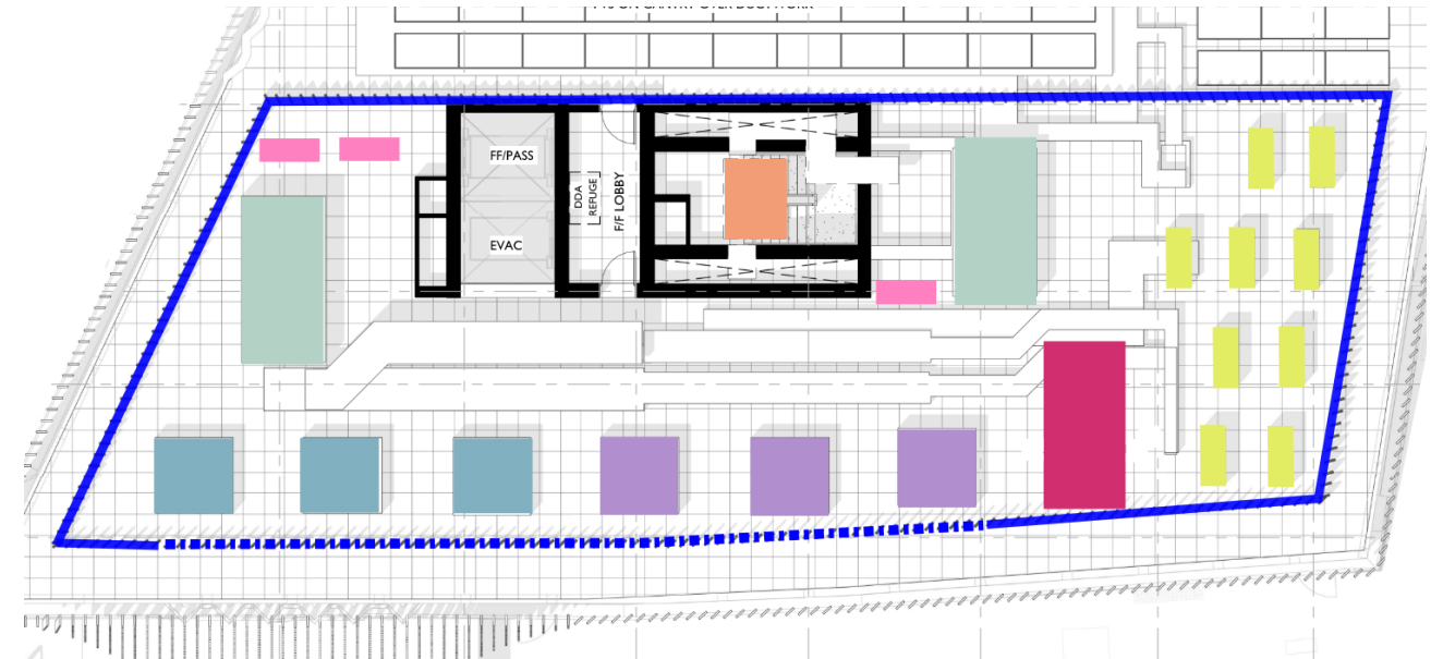
Figure 3 Preliminary roof plant layout
