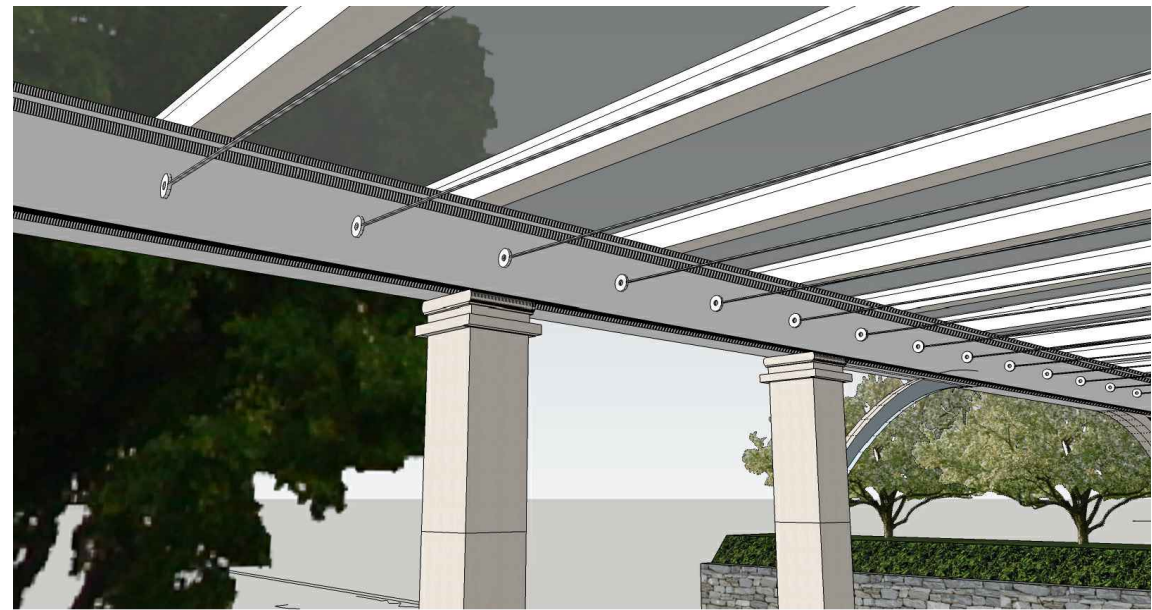
PORTE-COCHERE STRUCTURE: CONCEPT IMAGE SHOWING TENSILE CABLES FOR CLIMBING PLANTS & GLAZED ROOF FOR WEATHER PROTECTION
