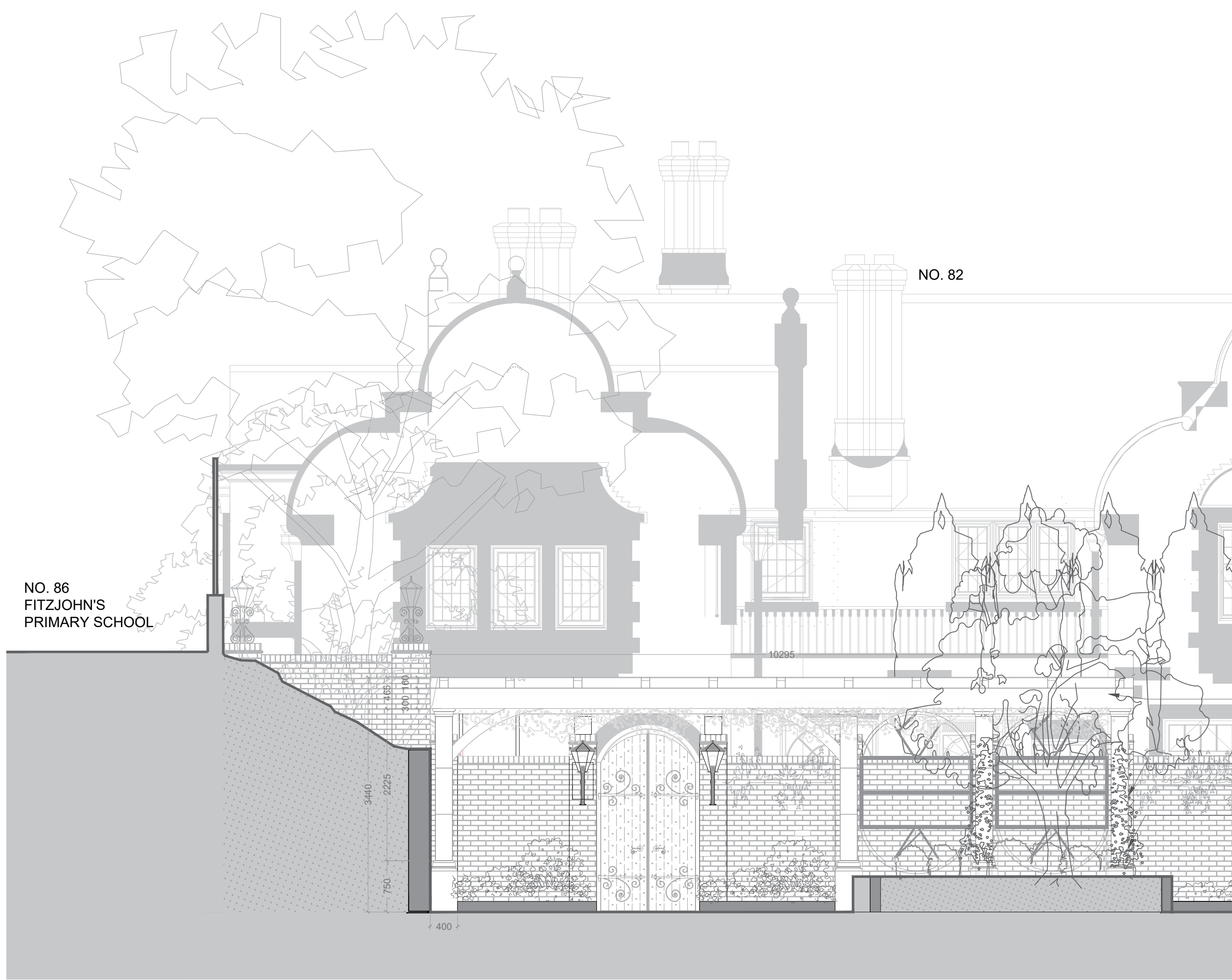
LA-046-013 PARTIAL SECTION C: Cross Section showing porte-cochere
