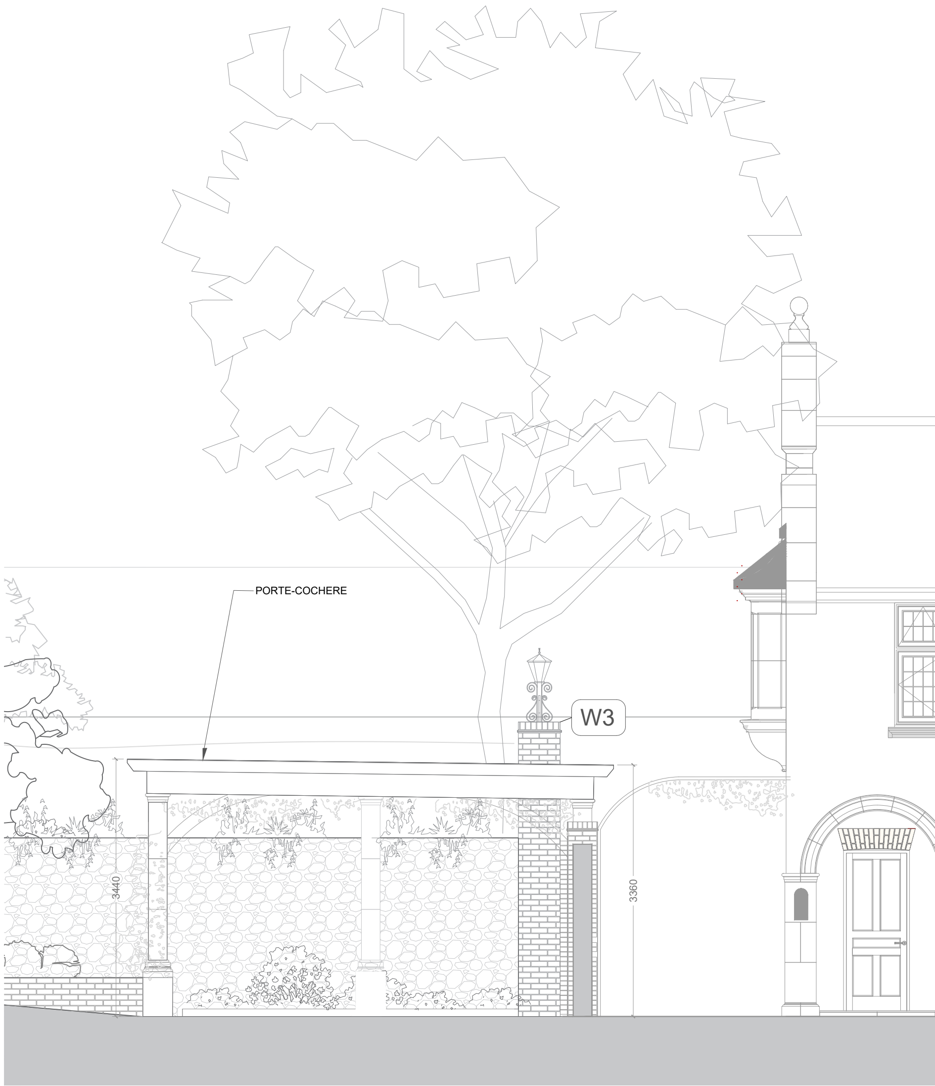
LA-046-013 PARTIAL SECTION B: Long Section showing porte-cochere
