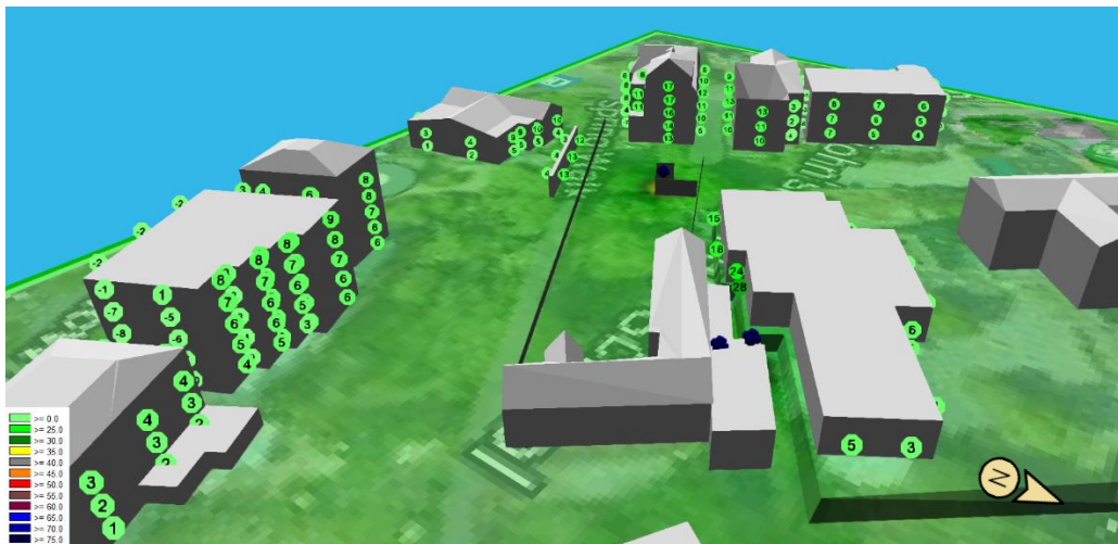
Figure 3: Condensing units CadnaA Noise Model (NIGHT TIME Attenuation Applied) View towards 84 Fitzjohn's Avenue
