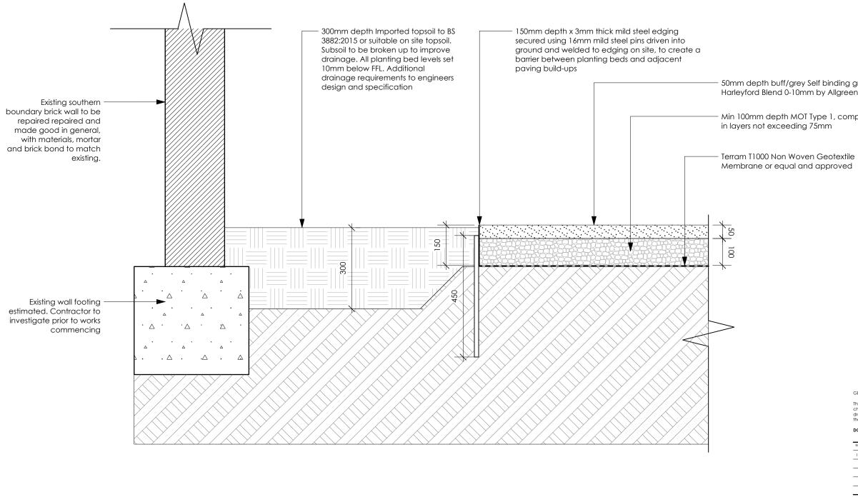
STEEL EDGING BETWEEN PLANTING BEDS AND SELF-BINDING GRAVEL BUILD-UP SECTION DETAIL
