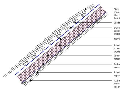
Strip existing tiles off roof, store, and relay once breather membrane has been installed. Where required, replacement tiles to match existing. Type to be approved by the council first. Relaid with nibs, matching existing. 25x38mm treated timber battens
