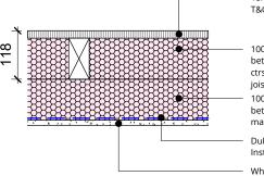
18mm moisture resistant chipboard loft panel T&G boards. Screw fixed into new ceiling joists.
