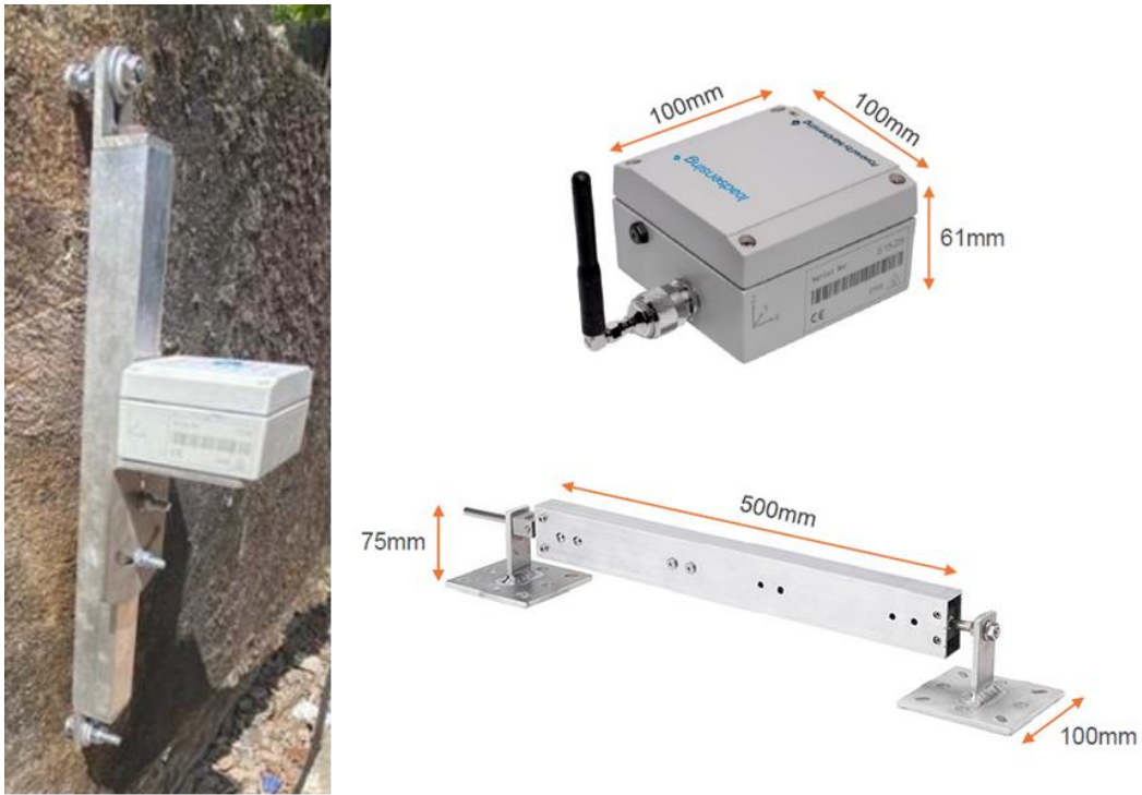
Figure 14 – Example of a tiltmeter
