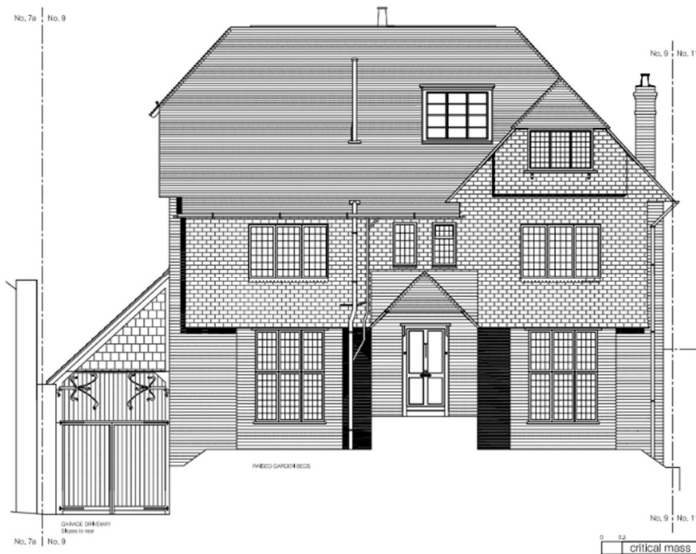
Existing elevation pre 2008 with modern dormer window and garage to left hand side.
