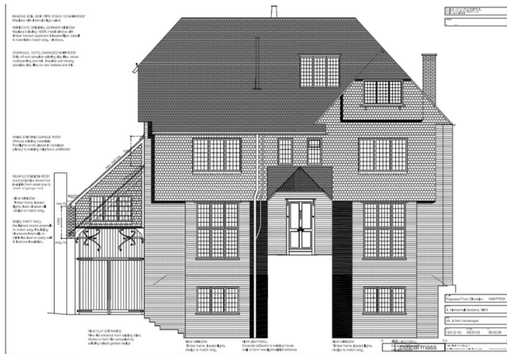
Proposed elevation 2008 to change dormer window to original Arts and Craft style and add study over garage.
