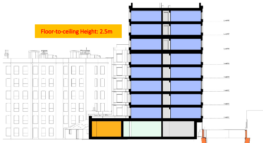
Figure E.1 – Early Design Section Showing Floor-to-ceiling Heights Produced by Sheppard Robson Architects
