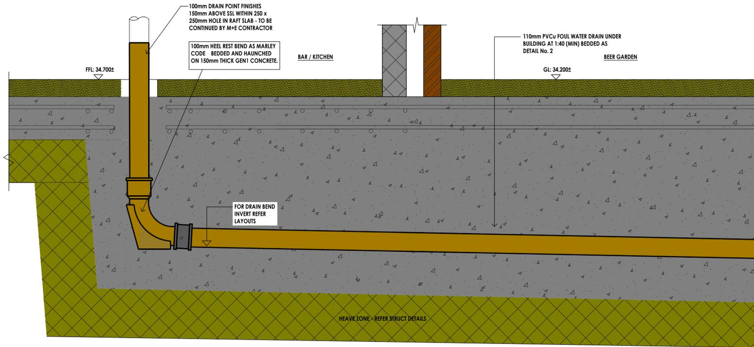
DETAIL No. 1 - INTERNAL DRAIN POINT UNDER RAFT
