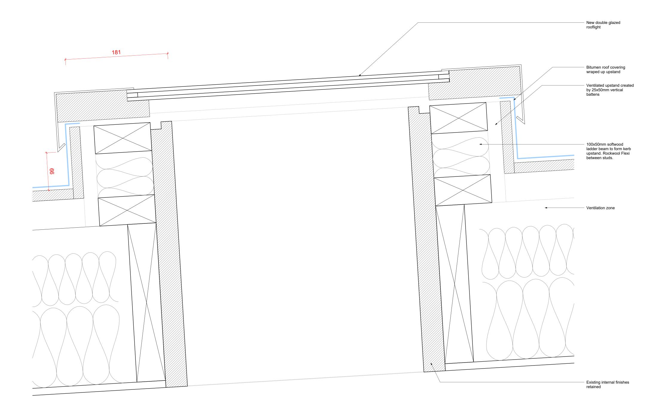
Proposed Rooflight - Typical Detail Section AA
