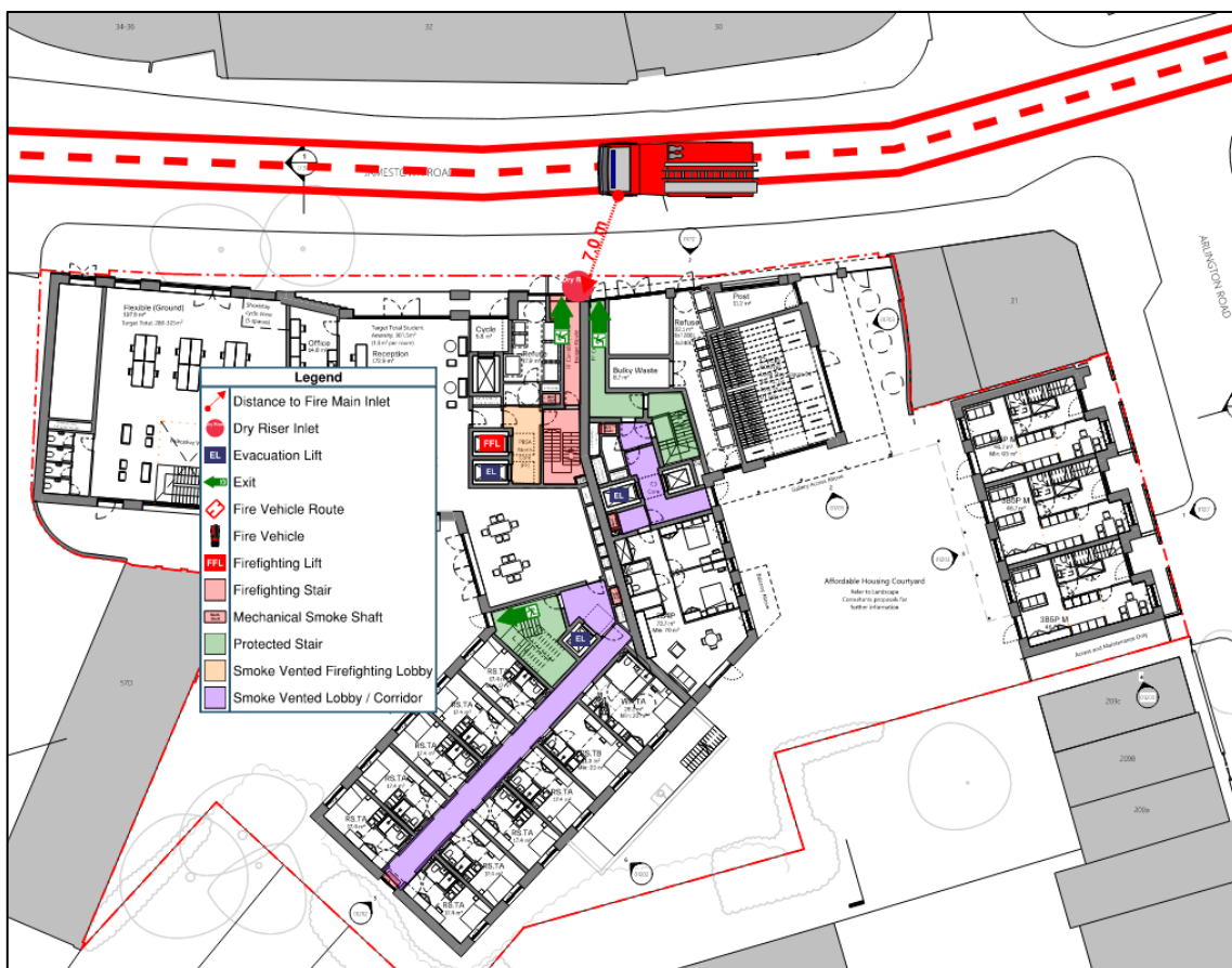
Figure 11: Fire Vehicle Access
