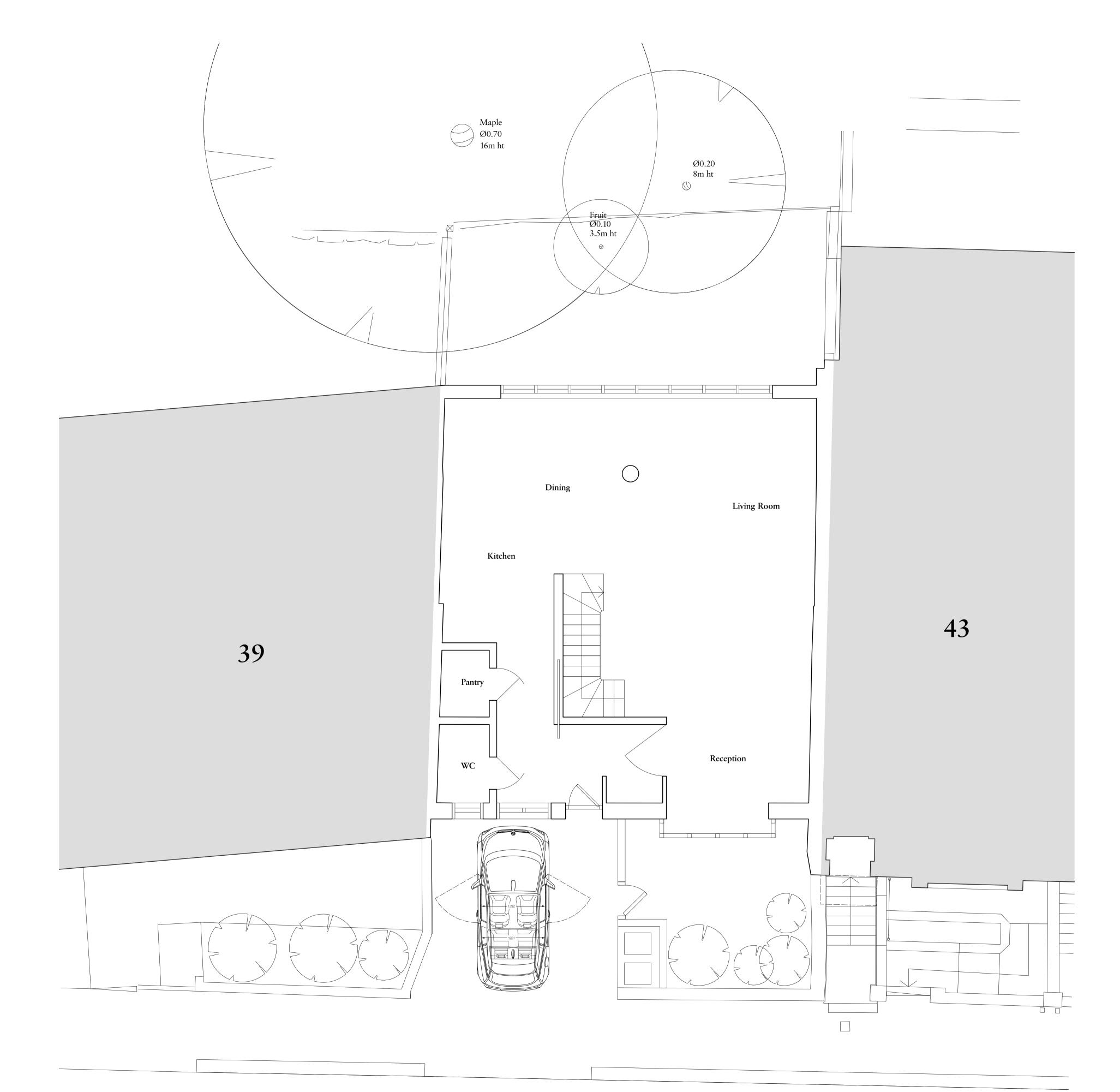
TREE SURVEY in accordance with the foreword of BS5837 2012: "Trees in relation to design, demolition and construction -Recommendations" which specifes the information required for a full tree survey and which is provided on this plan
