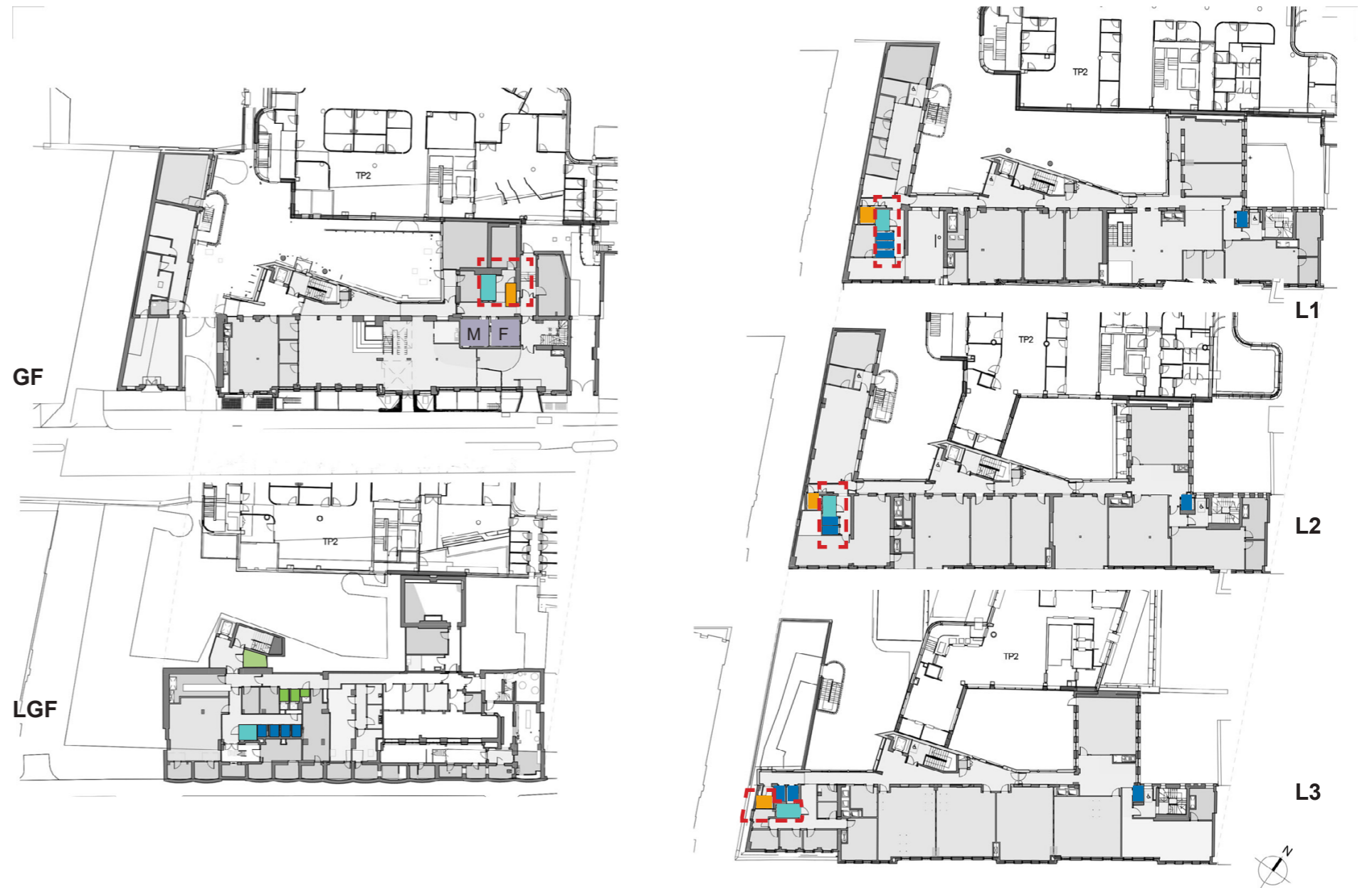
WC and shower distribution
