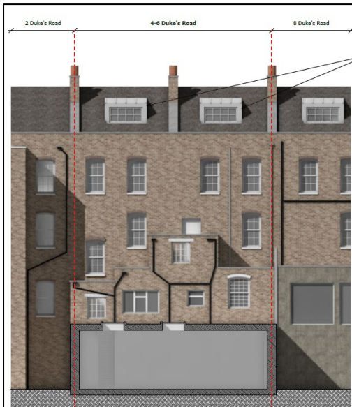
Proposed rear elevation showing the proposed new dormers on both roof slopes.
