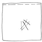
PLANE TOP OF BEAM SMOOTH AND FLAT TO RECEIVE STEEL PLATE (MAX. 3mm DEPTH).
