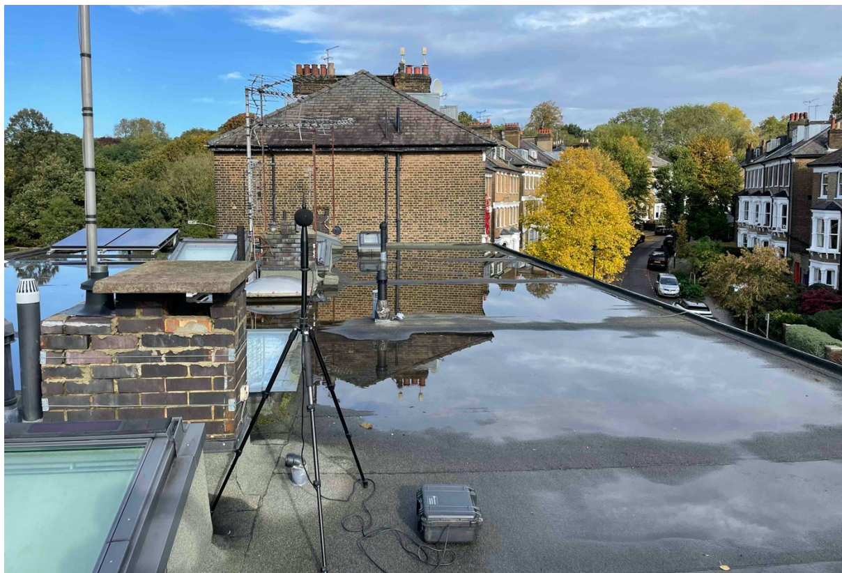
Figure 5: Noise survey equipment on roof of 80-90 South Hill ark
