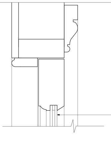
12MM SLIMLINE GLAZING: •4MM SOFTCOAT 1.1 •4MM ARGON FILLED CAVITY •4MM CLEAR =U-VALUE 1.2 W/m2K
