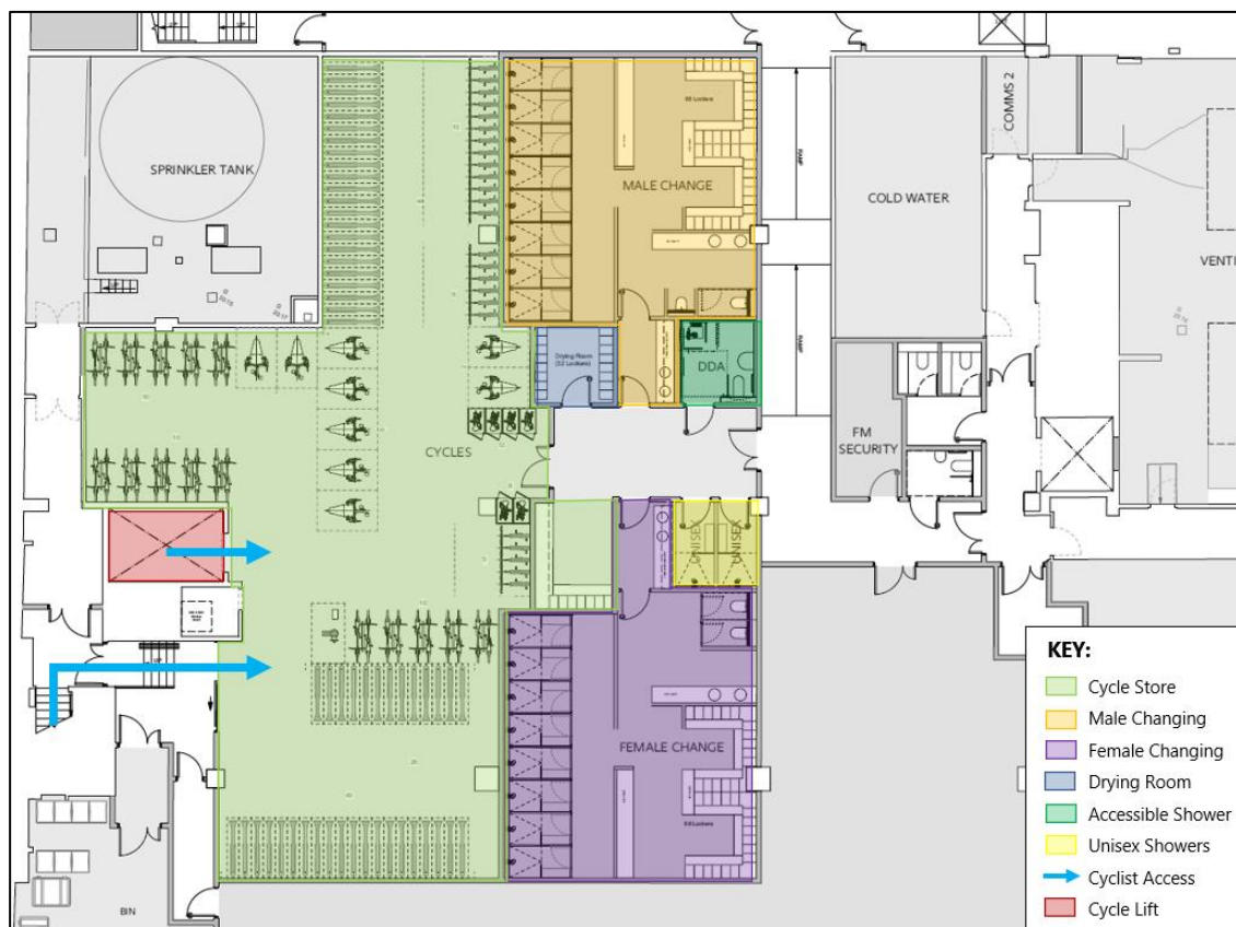
Figure 5.3: Basement – Cycle Parking Arrangement Source: Stiff+Trevillion Architects 2024
