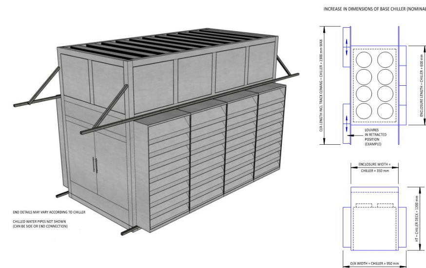
Figure 3 Example acoustic enclosure for ASHPs, (Source: Allaway Acoustic's AA301S)
