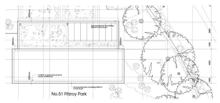
The original planning drawings indicate that the upper roof section is approximately 13m in length and approximately 5.5m in width. With a row spacing of 1508mm, 18, Q-peak-duocell 410 modules would be installed, the panel size is 1879mm x 1045mm x 32mm.
