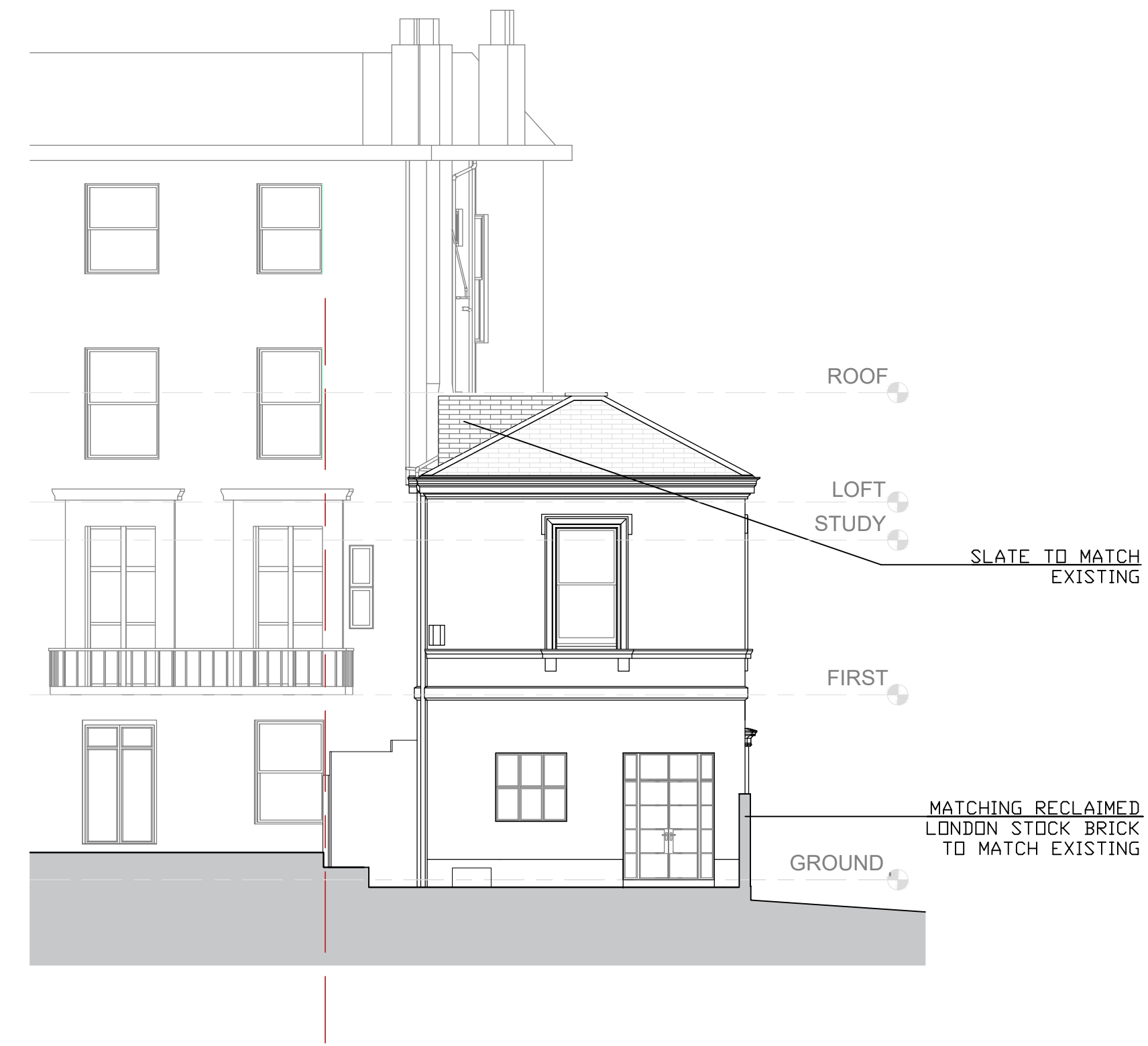
2. EAST ELEVATION 1:100 (SIDE)
