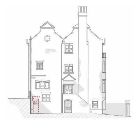
This application proposes to amend an existing high level window on Lower Ground Floor level to form a new side entry door to the existing west facing side elevation to 5 Cannon Place.
