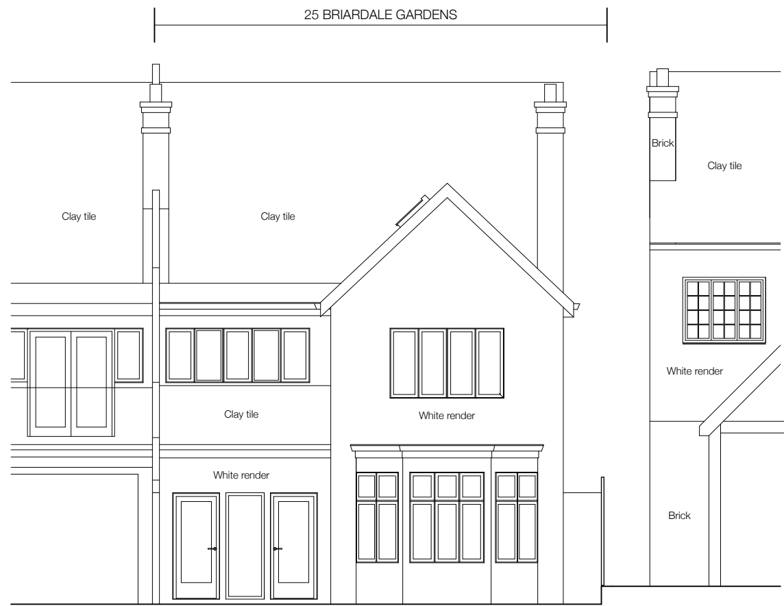
EXISTING FRONT ELEVATION
