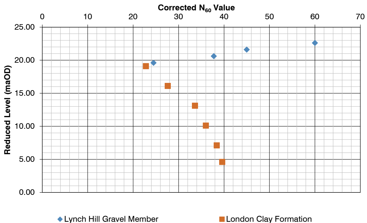
Figure 3.4.1 Corrected N 60 Values vs. Depth
