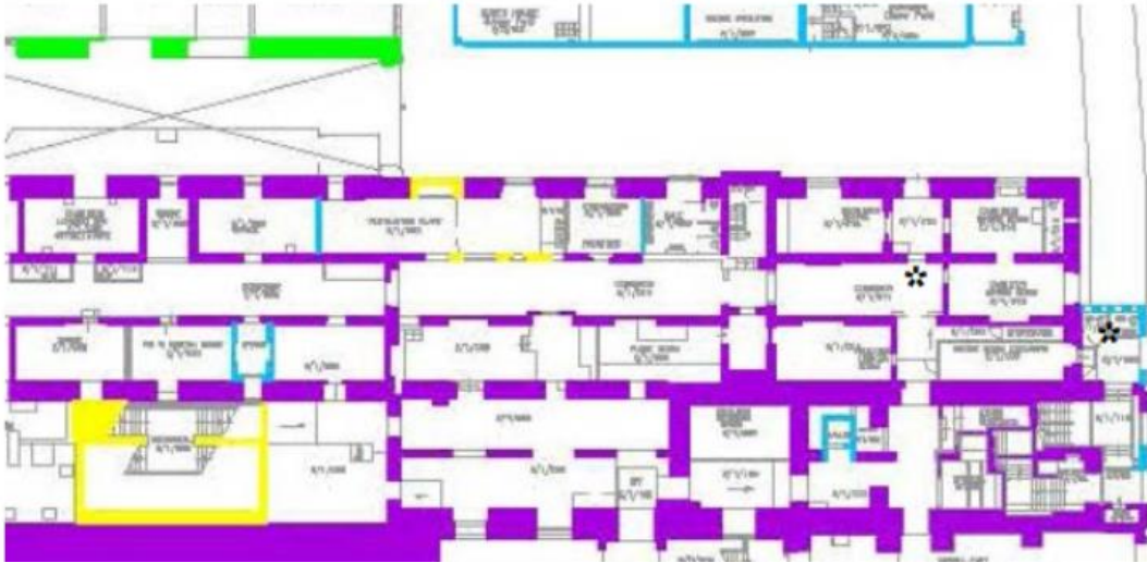
Figure 2. Extract from the CMP significance plans. Purple is 'very high' significance; light blue is 'low significance'. Areas of alteration are marked with an asterisk.
