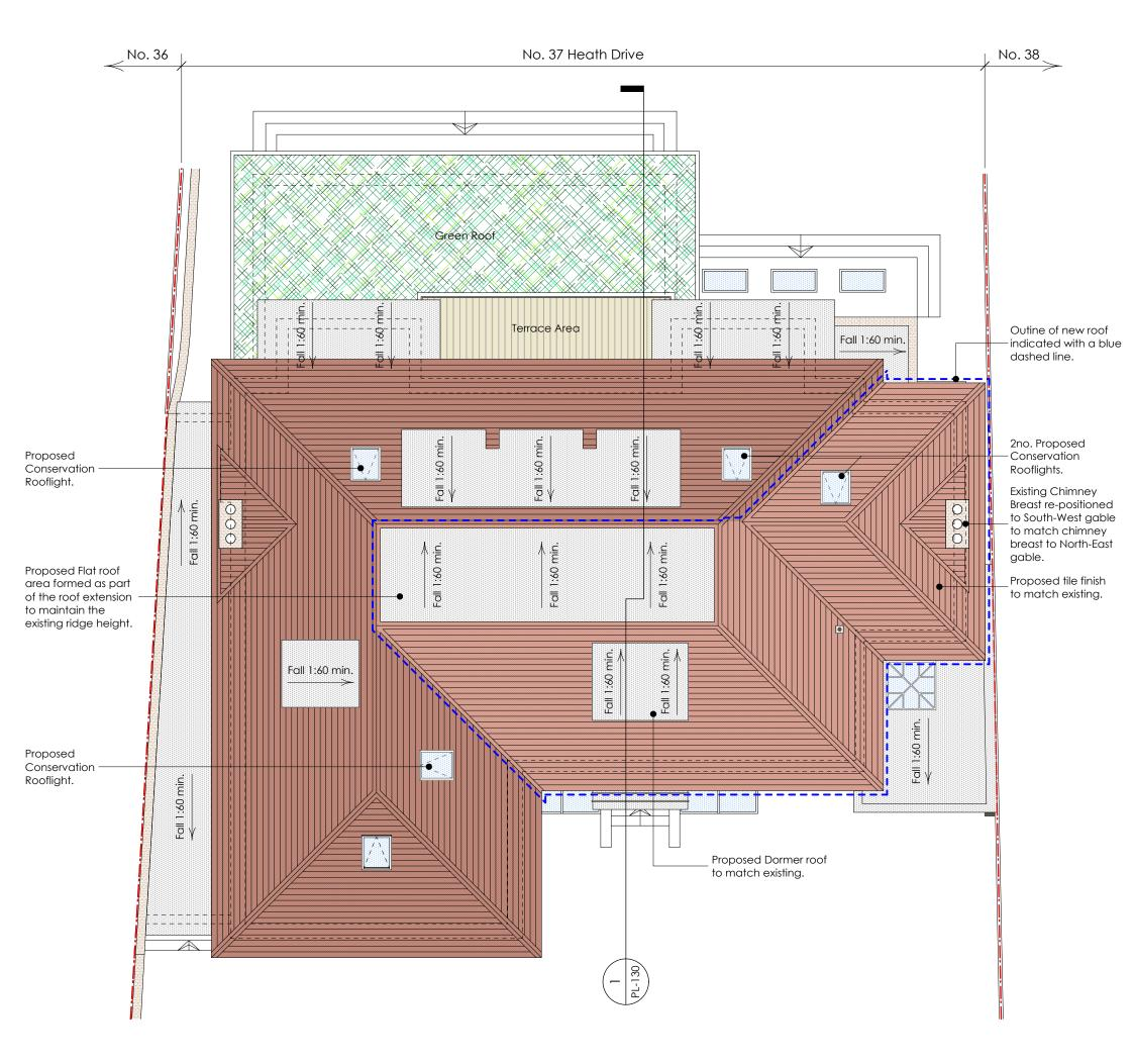
**Proposed Roof Plan** scale: 1:100 @ A3
