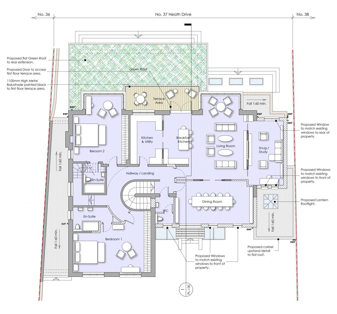
**Proposed First Floor Plan** scale: 1:100 @ A3
