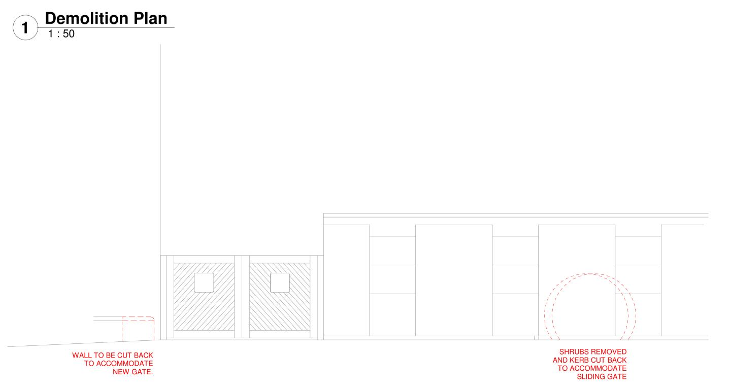
**Demolition External Elevation - North**1:50
